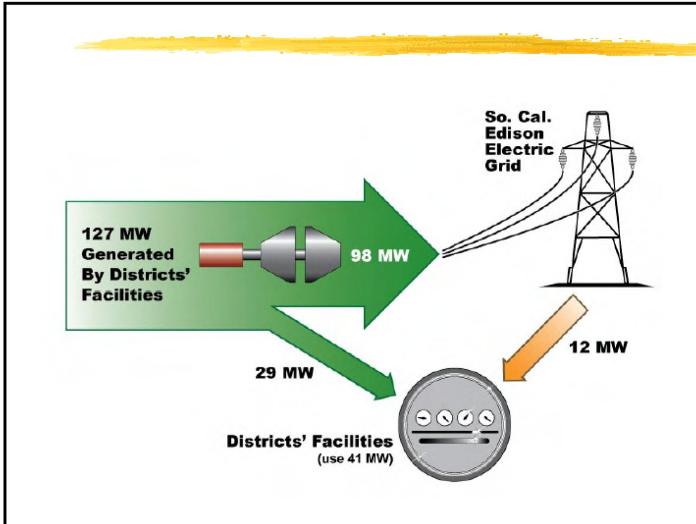
From "The Power of Digester Gas: A Technology Review from Micro to Megawatts,"
