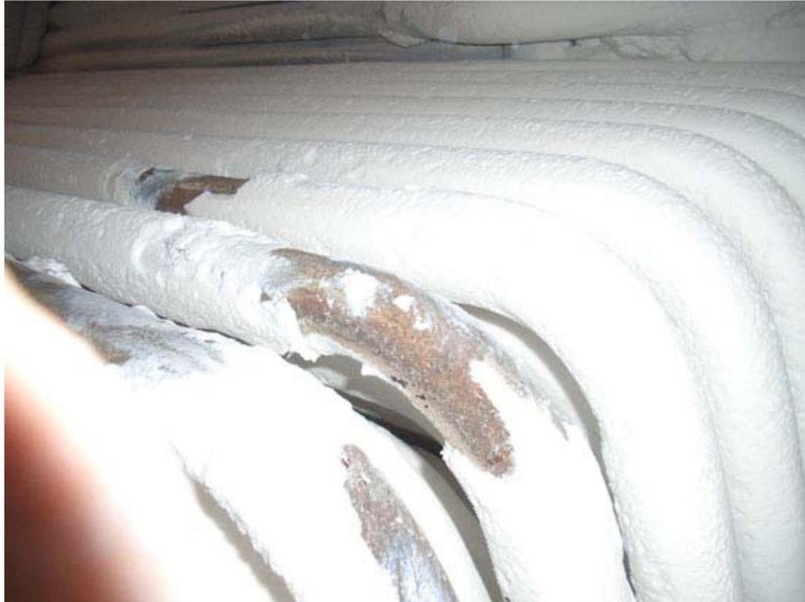
**The sand-like material is  $\text{SiO}_2$  produced through oxidation (burning) of the volatilized siloxanes contained in the digester gas. Figure shows siloxane deposition on boiler tubes.**
