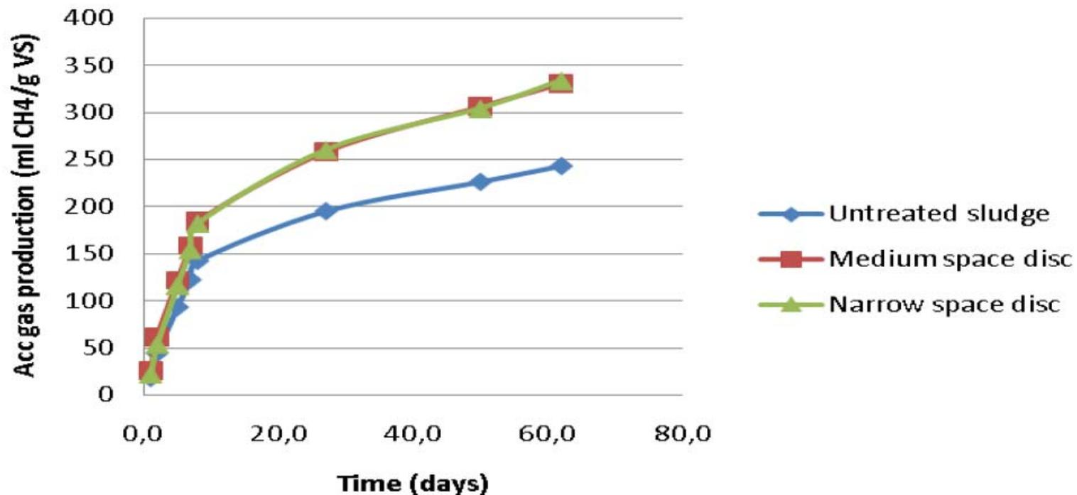
**Specific methane production of biological excess sludge (DS content 5.7%, VS content 3.7%) treated with the Krima disperser narrow spaced disc and medium spaced disc respectively**
