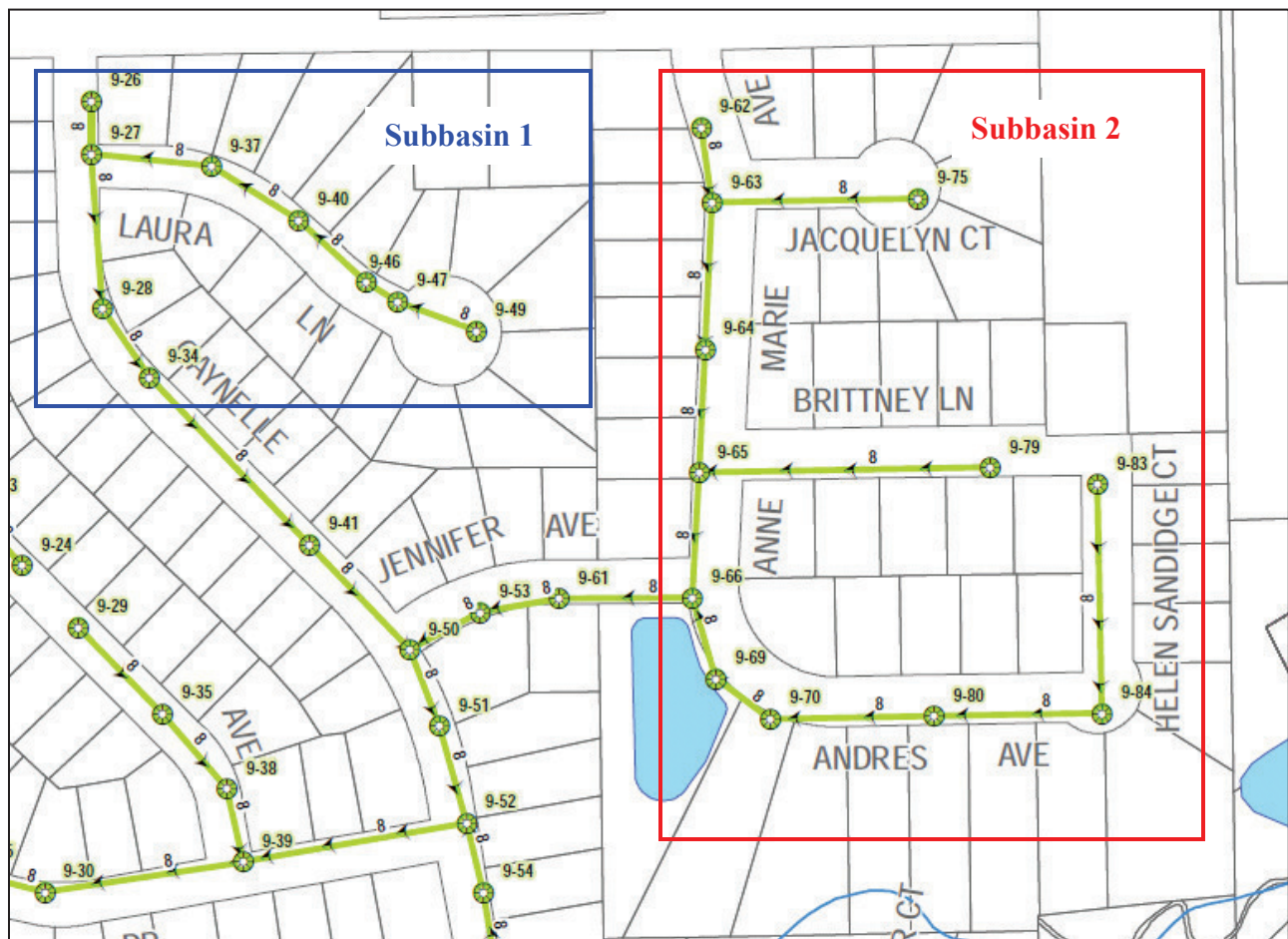
Figure 8.3. Subbasins Tributary to the Same Sanitary Main Line (Courtesy of the Village of Tinley Park)
