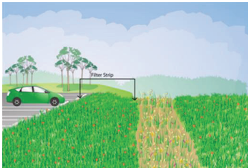
Figure 5.19. Illustration of a Filter Strip
