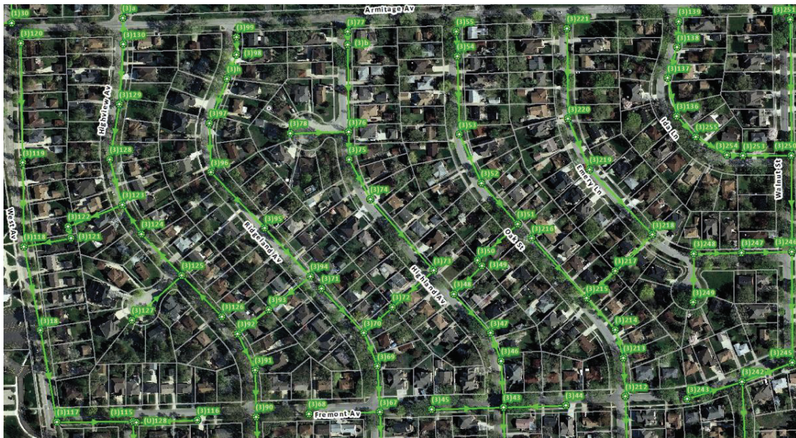
Figure 8.16. GIS-Based Sewer System Mapping
