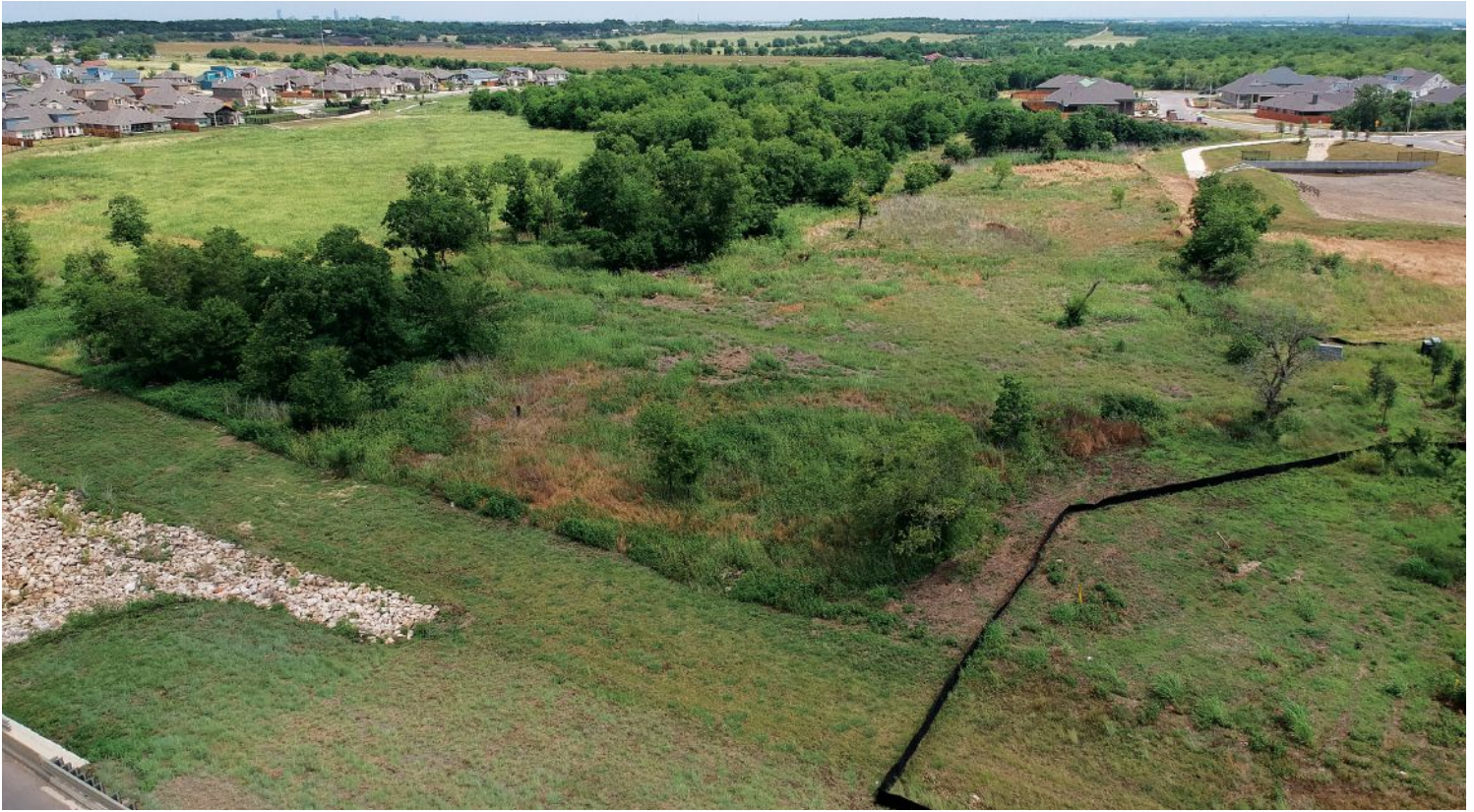
A network of seepage berms promotes infiltration and reduces storm water erosion.
