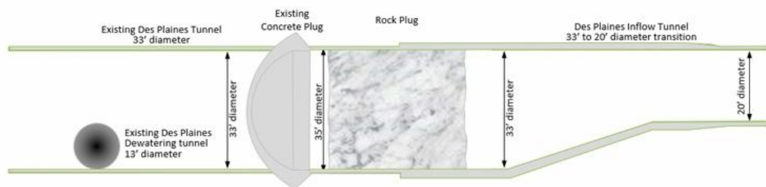
The Des Plaines Tunnel transitions from 33 feet in diameter to 20 feet, where it will connect from the inflow tunnel to the McCook Reservoir.
