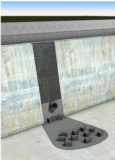
The 20-foot-diameter Des Plaines Inflow Tunnel will spill on to the reservoir. Concrete blocks slow the force of water.
