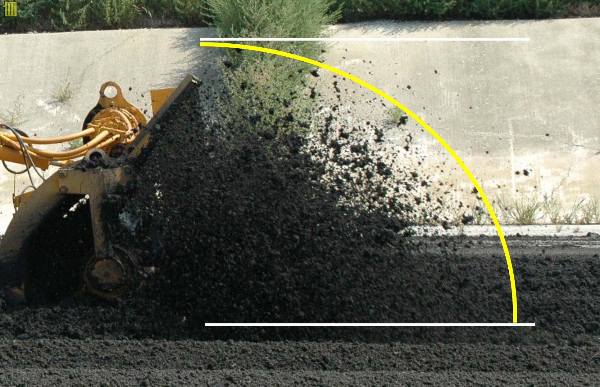
**(Paddle Aerator) During Air-Drying On Paved Drying Cells**
