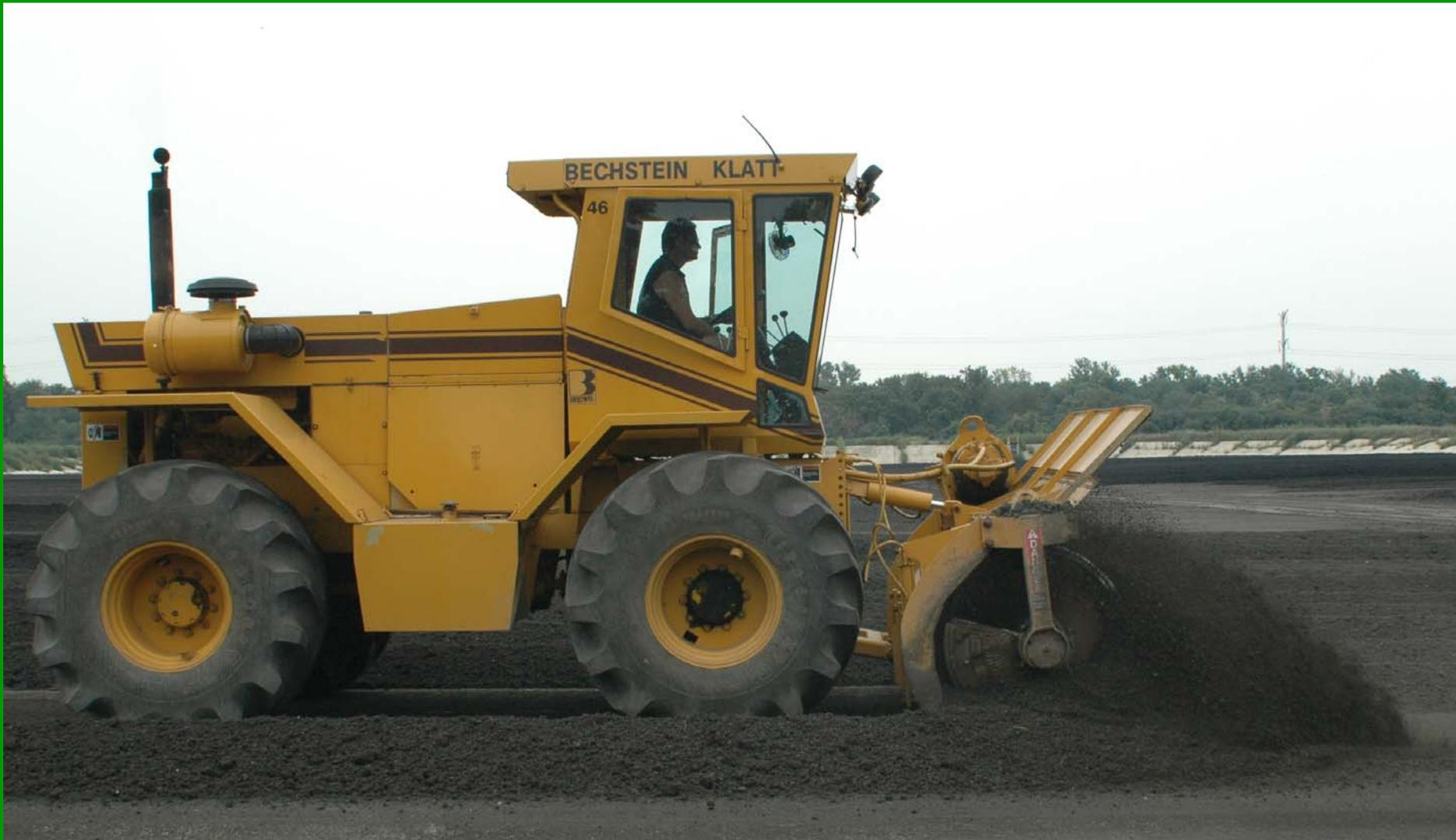
**Biosolids Mechanically Agitated (Auger) During Air-Drying On Paved Drying Cells**
