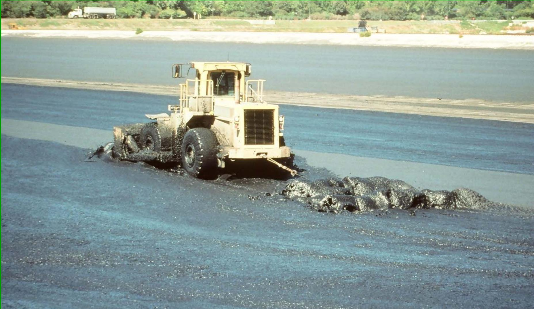
**Rail System Pulled by a Bulldozer On Paved Drying Cells**
