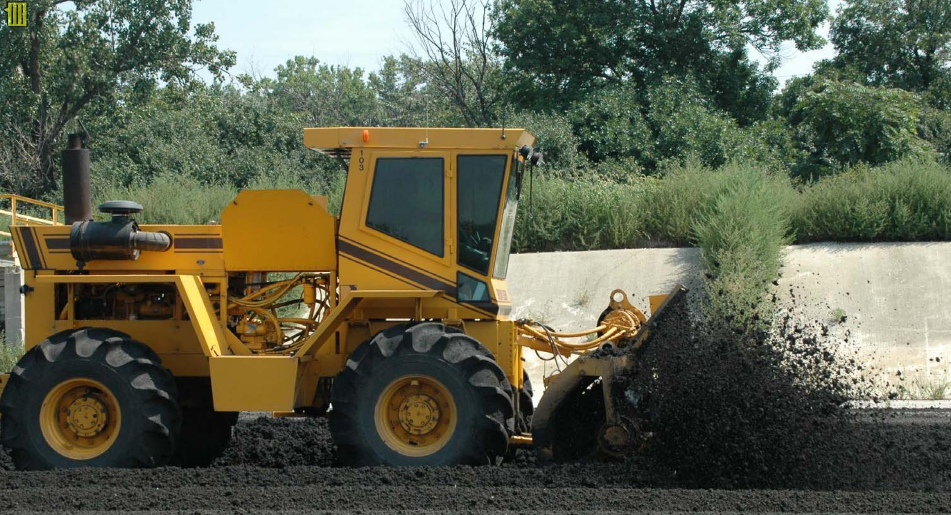
**Biosolids Mechanically Agitated (Paddle Aerator) During Air-Drying On Paved Drying Cells**
