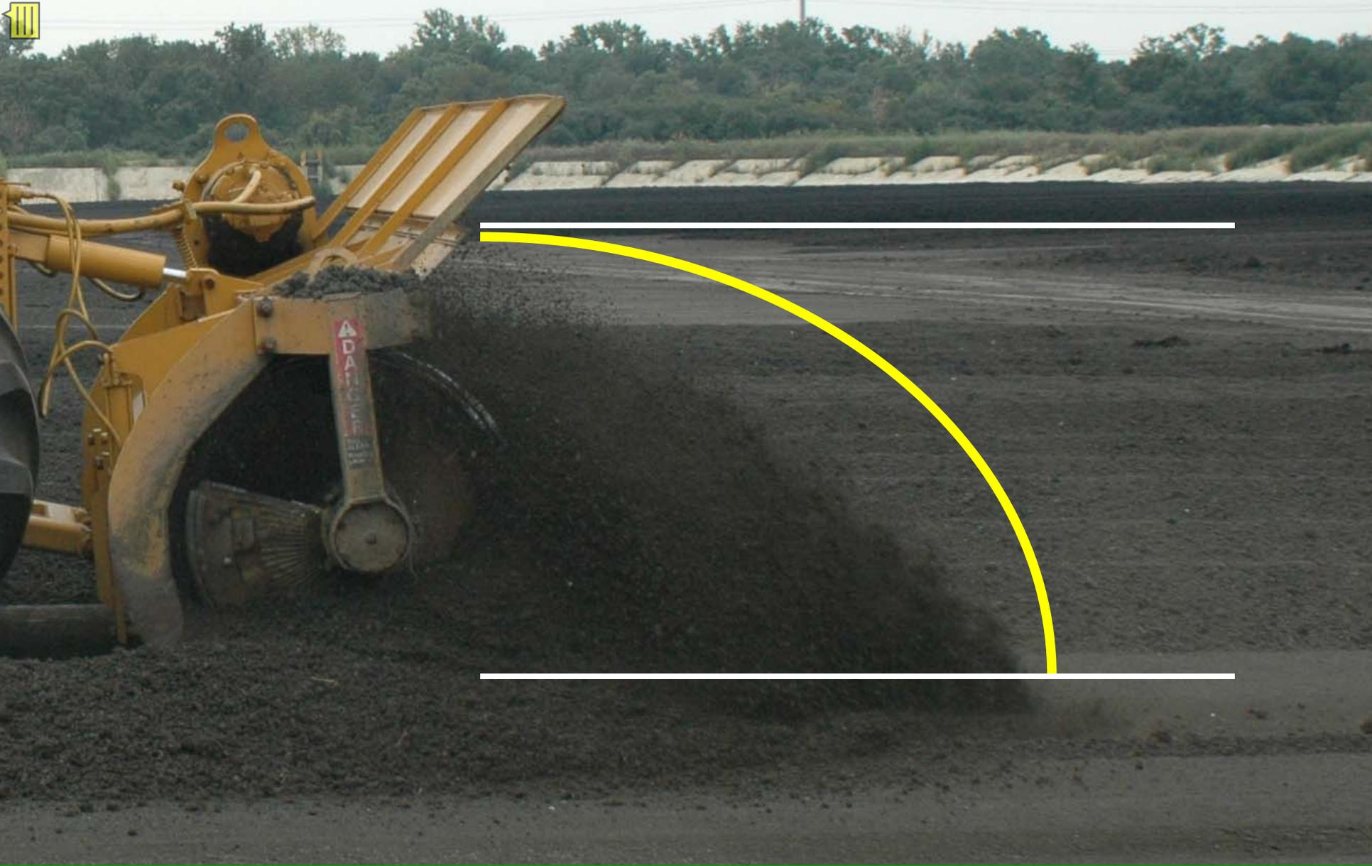
**(Auger) During Air-Drying On Paved Drying Cells**
