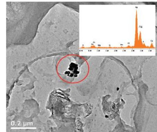
FIGURE 4. TEM image of colloidal material from sock 1a washwater. Inset: EDX confirmation that the dark particles within the circle are predominantly silver.
