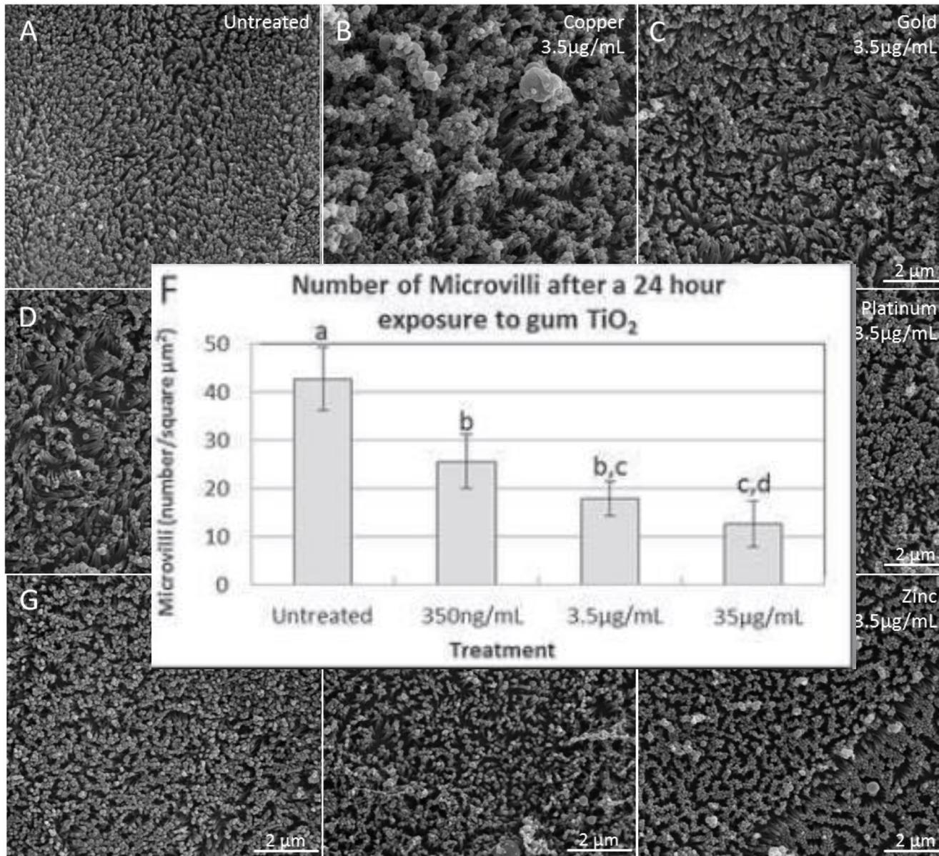
Figure 4. SEM images of microvilli exposed to  $1 \mu\text{g}/\text{cm}^2$  NMs ( $3.5 \mu\text{g}/\text{mL}$ ), except “A”, which is an untreated control. After exposure to NMs from supplement drinks, both the normal organization and the number of microvilli changed compared to untreated controls. Large spherical particles ( $>250 \text{ nm}$ ) are membrane blebs.
