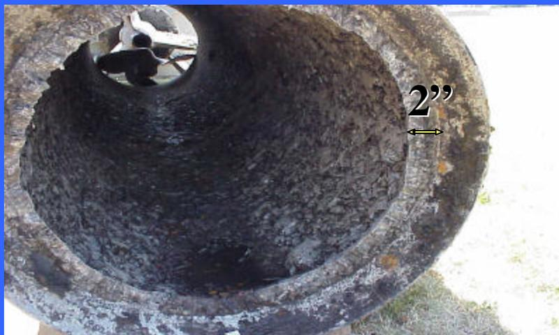
Pipe clogging and scale formation in anaerobic digesters
