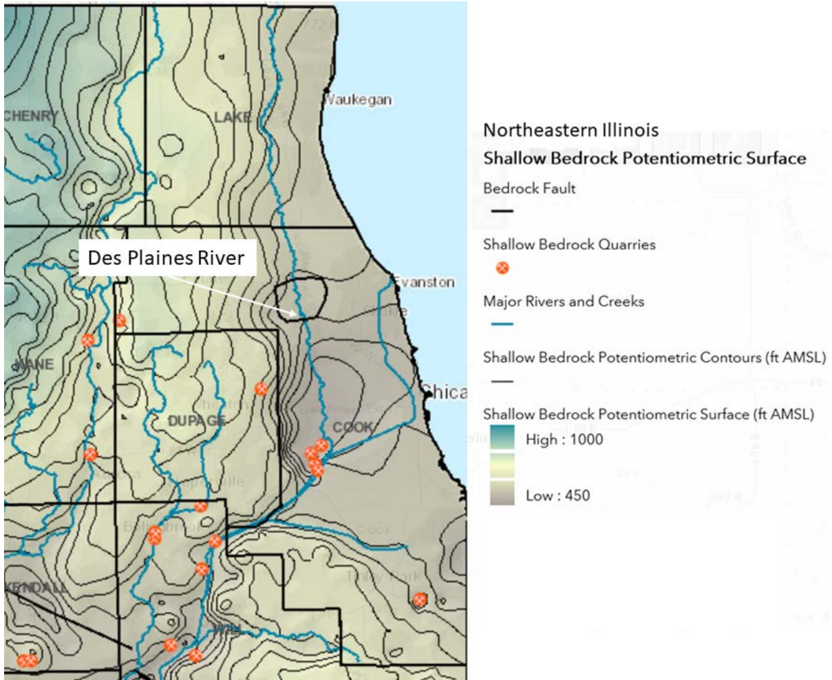
Figure 3.6-5 Shallow Bedrock Potentiometric Surface in Northeastern Illinois Source: Illinois State Water Survey, Prairie Research Institute
