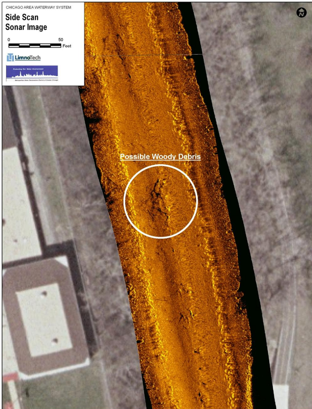
Figure 3-3: Example of Side Scan Sonar Imagery from the CAWS, Overlain on Aerial Imagery (Imagery Collected in Upper North Branch of the Chicago River).
