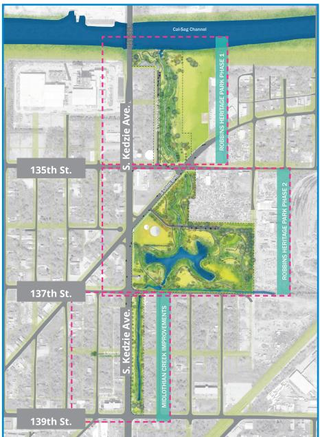
pond will be constructed east of Kedzie between 135th and 137th streets and north of Midlothian Creek. The Robbins Stormwater Park will allow for a naturalized wetland detention area along with channel improvements to resemble a park-like setting in central Robbins. Bioswales will be planted along Spaulding and Sawyer Avenues
