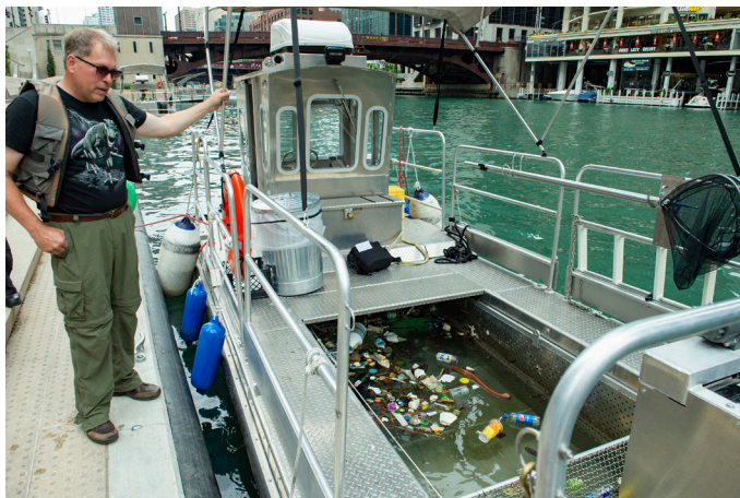
MWRD staff remove plastic trash and other debris from the main stem of the Chicago River. The fleet of skimmer boats operate along the Chicago area waterways from mid-April to mid-October, and after significant storms year round, unless weather conditions prohibit safe operations. A basket kept at water level collects debris as the boat trolls over it. A larger MWRD debris boat operates year-round with a crane to lift heavier materials.
