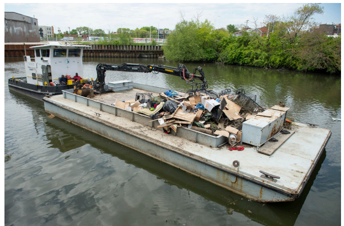
MWRD staff remove plastic trash and other debris from the main stem of the Chicago River. The fleet of skimmer boats operate along the Chicago area waterways from mid-April to mid-October, and after significant storms year round, unless weather conditions prohibit safe operations. A basket kept at water level collects debris as the boat trolls over it. A larger MWRD debris boat operates year-round with a crane to lift heavier materials.
