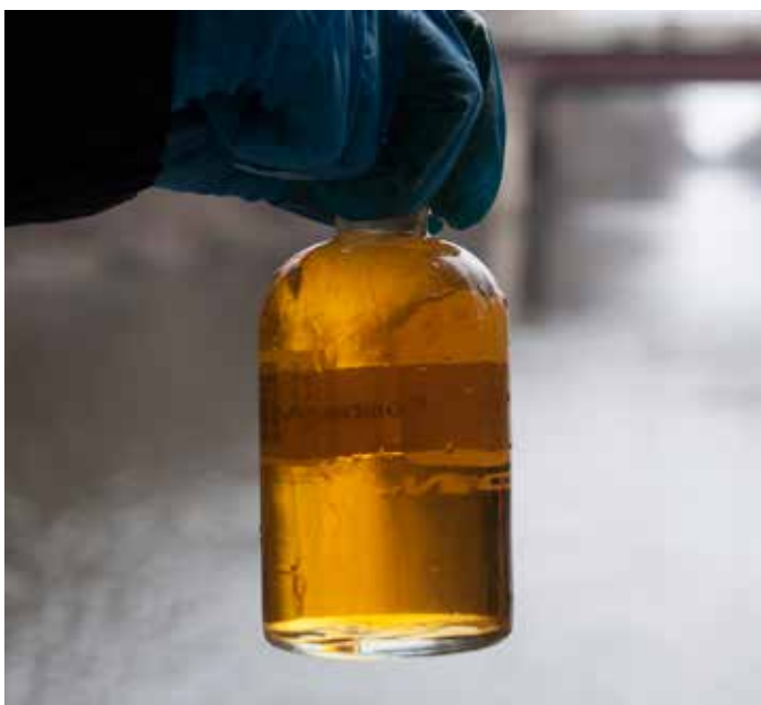
Top left: A water quality meter is retrieved from its stainless steel housing on the Main Stem of the Chicago River and is replaced with a clean, calibrated meter. Top right: A probe is used to take waterway dissolved oxygen readings to compare to the readings taken by the instrument deployed in the field. Bottom left: A water sample is prepared for dissolved oxygen analysis on the North Branch of the Chicago River. Bottom right: Water samples are analyzed for ammonia in an analytical lab at the District's Stickney Water Reclamation Plant.
