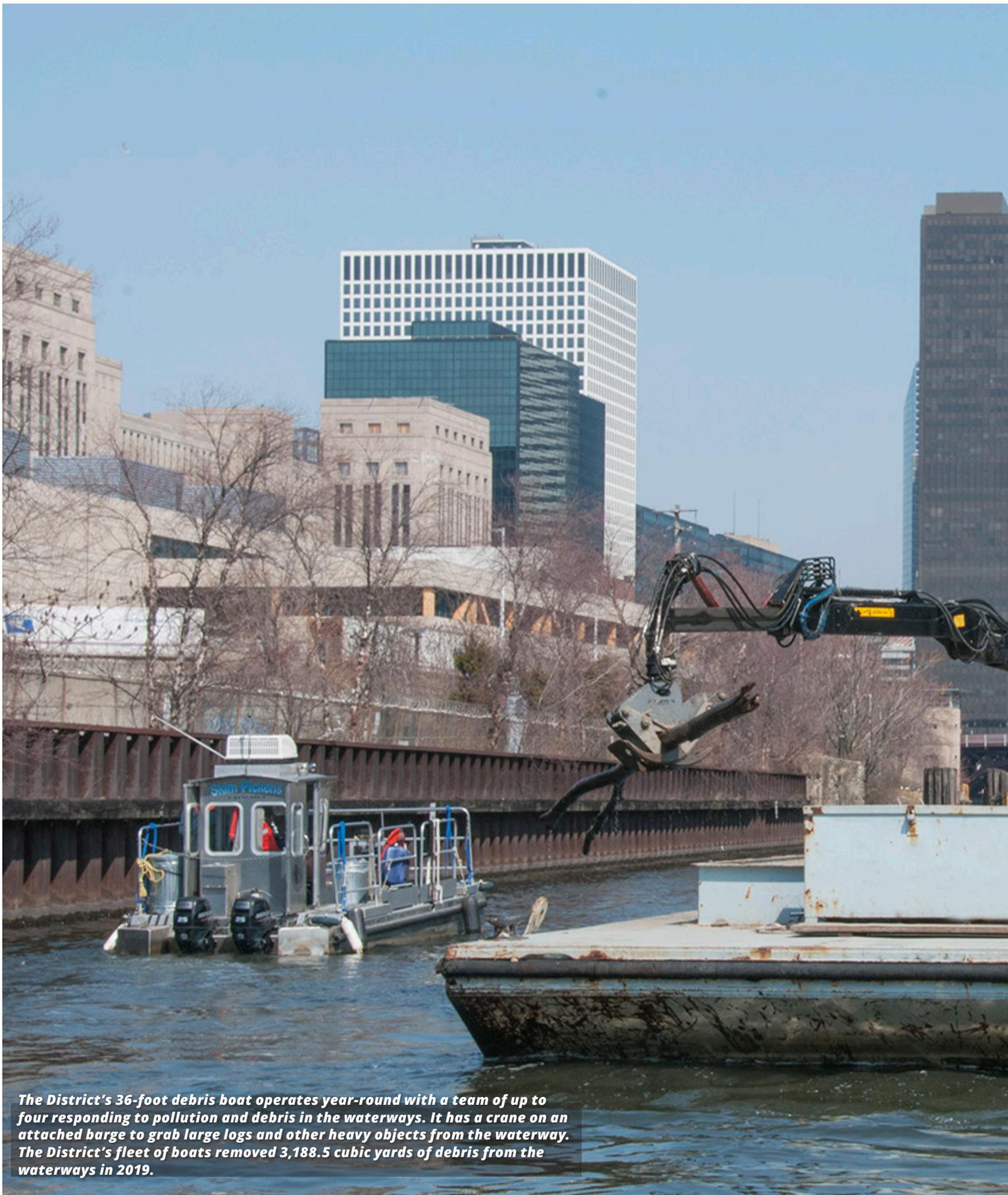
*The District's 36-foot debris boat operates year-round with a team of up to four responding to pollution and debris in the waterways. It has a crane on an attached barge to grab large logs and other heavy objects from the waterway. The District's fleet of boats removed 3,188.5 cubic yards of debris from the waterways in 2019.*
