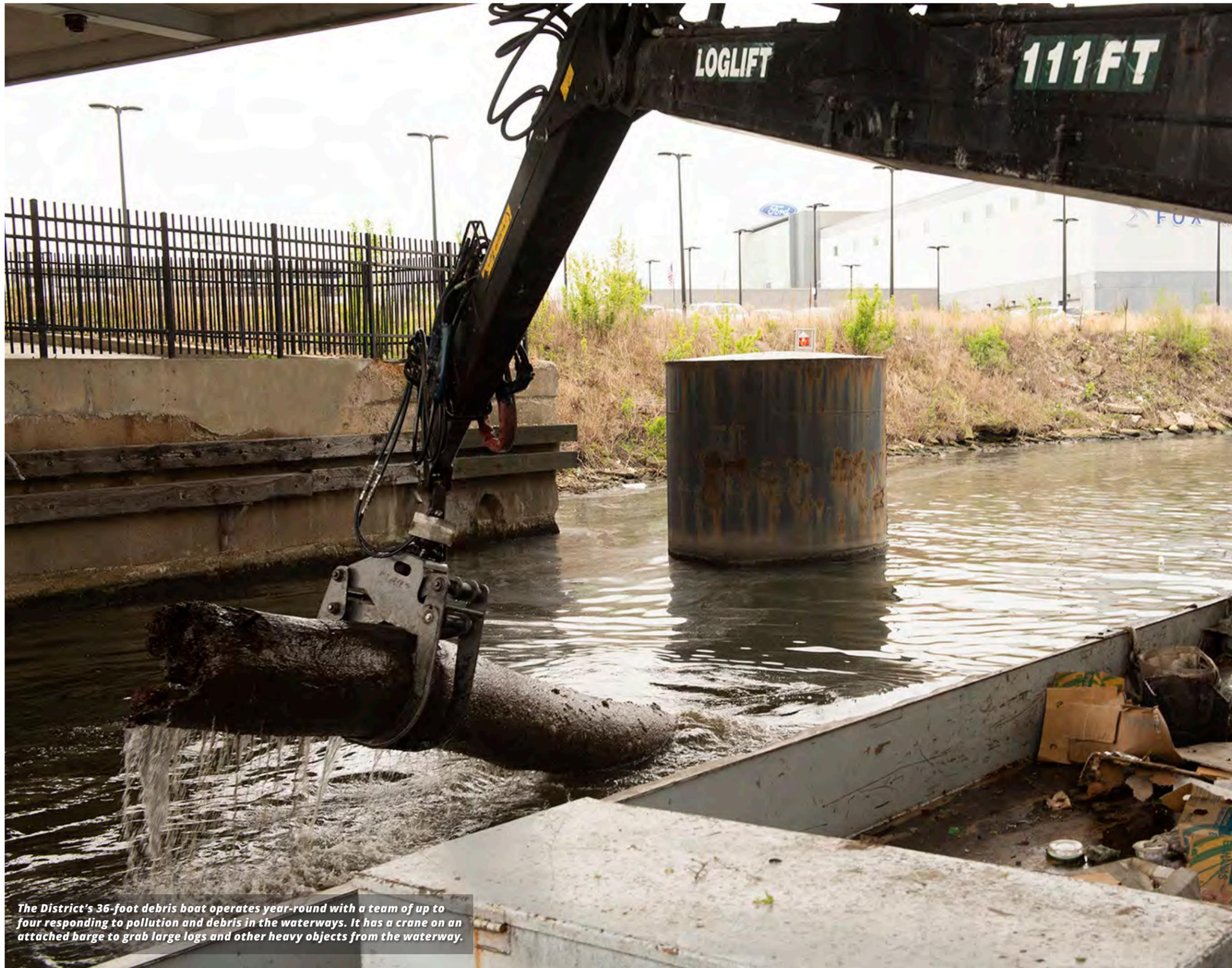
*The District's 36-foot debris boat operates year-round with a team of up to four responding to pollution and debris in the waterways. It has a crane on an attached barge to grab large logs and other heavy objects from the waterway.*
