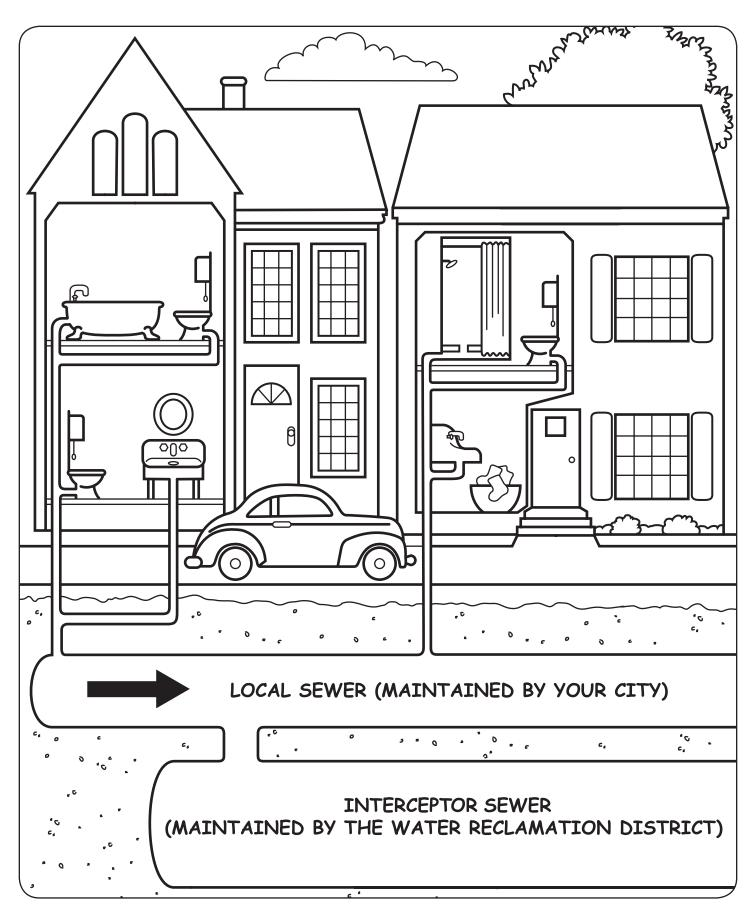
Every time you turn on the faucet or flush your toilet, the water goes down the drain into a local sewer. The water then goes to an intercepting sewer, where it travels to the District's treatment plants. The first plant was built in the 1920s.
