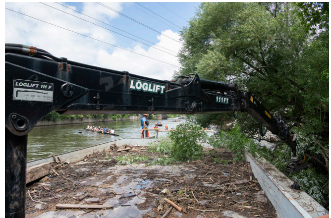
A crane on the MWRD's debris boat lifts trash, logs and other large objects that block the Chicago Area Waterway System (CAWS). The 36-foot boat is equipped with a 25-foot by 50-foot barge that patrols all 76 miles of the CAWS, year-round.
