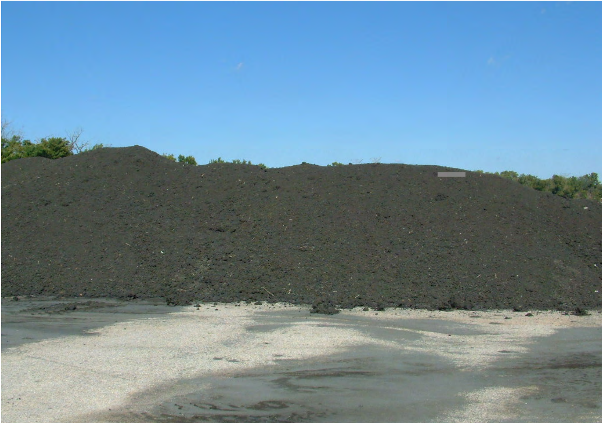
Air-Dried Biosolids Stacked for Transport to Beneficial Use Sites
