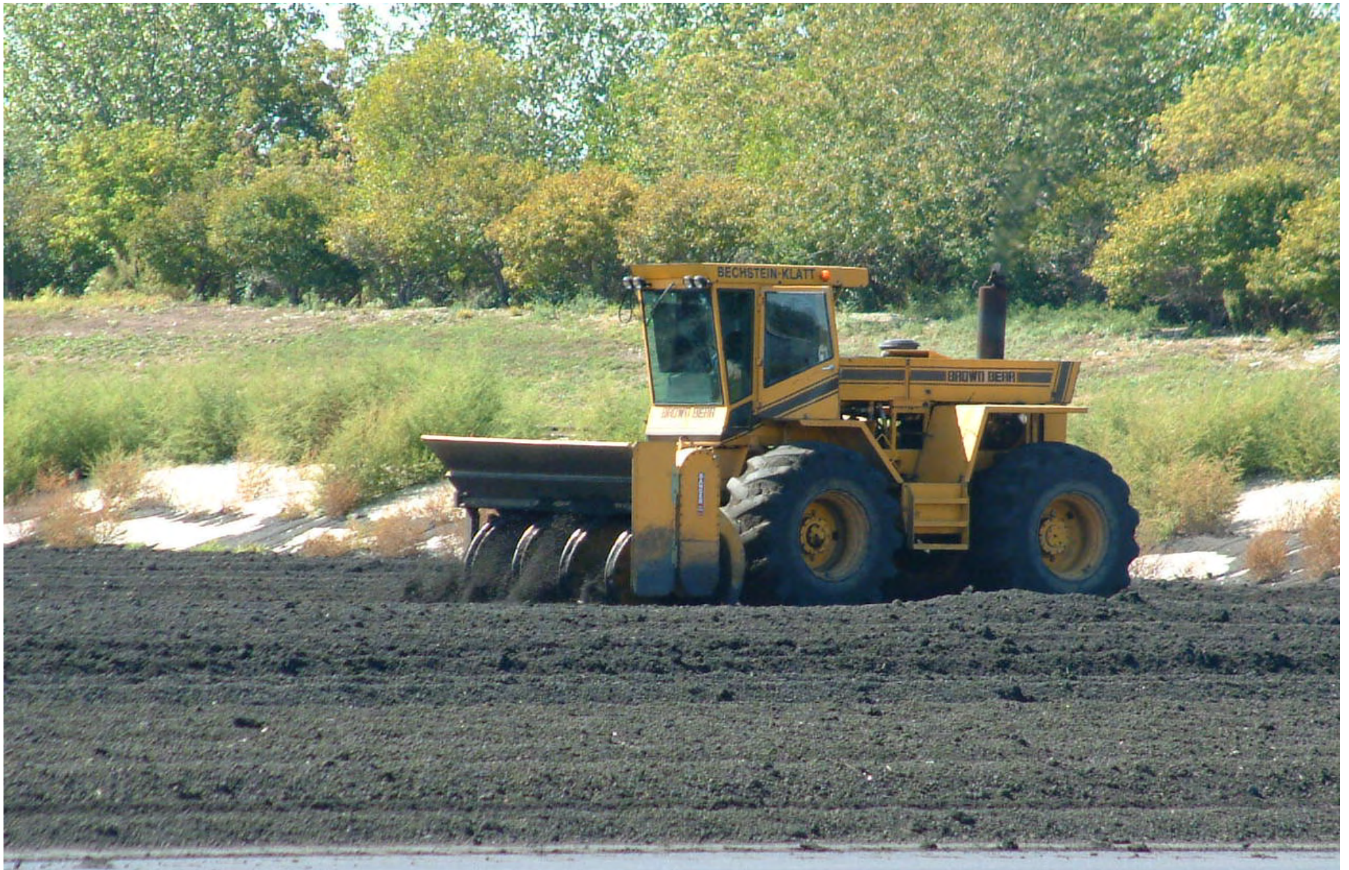
Lagoon-Aged Biosolids Being Mechanically Agitated During Air-Drying On Paved Drying Cell At SWRP HASMA Facility
