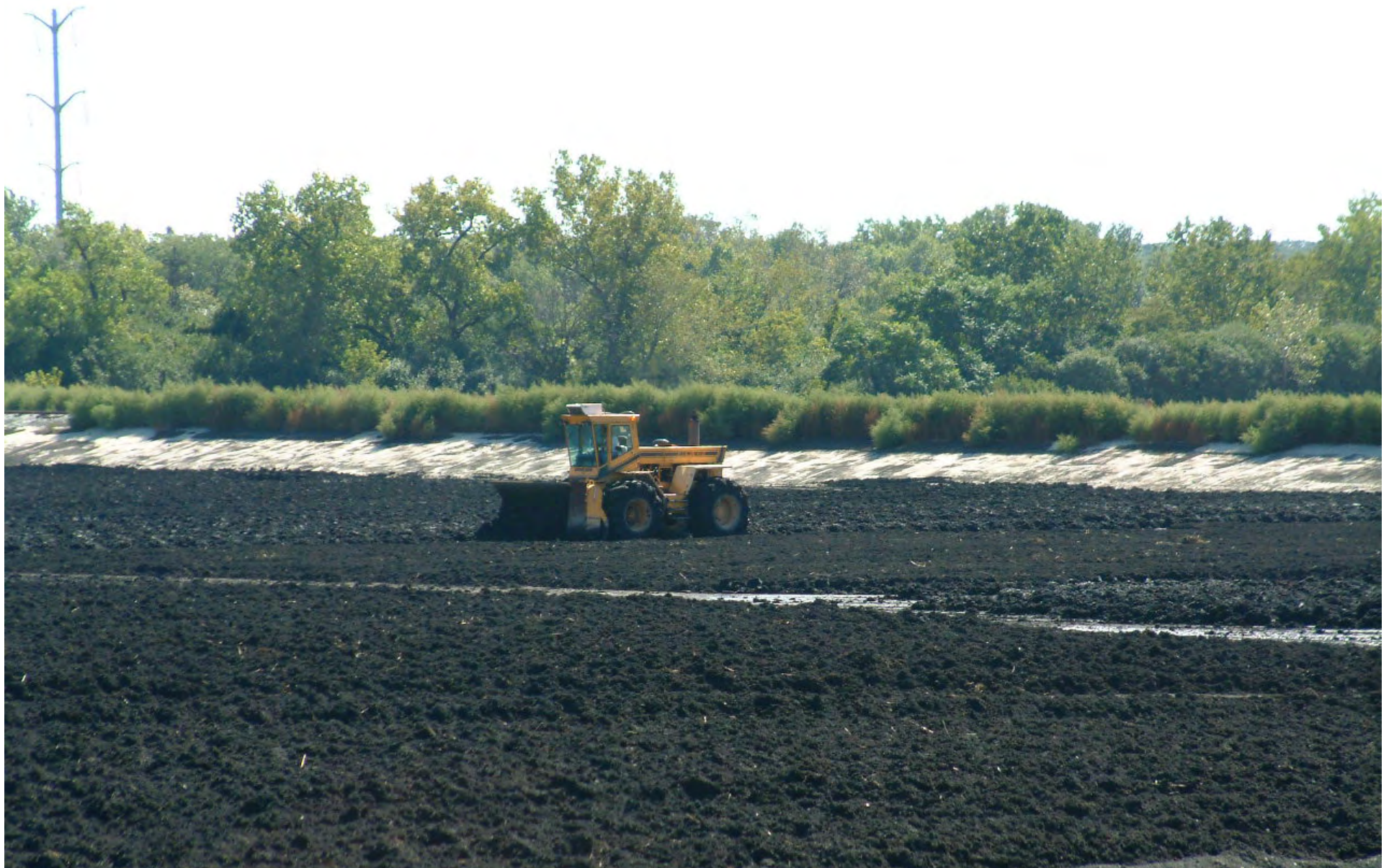
Lagoon-Aged Biosolids Being Mechanically Agitated During Air-Drying On A Paved Drying Cell
