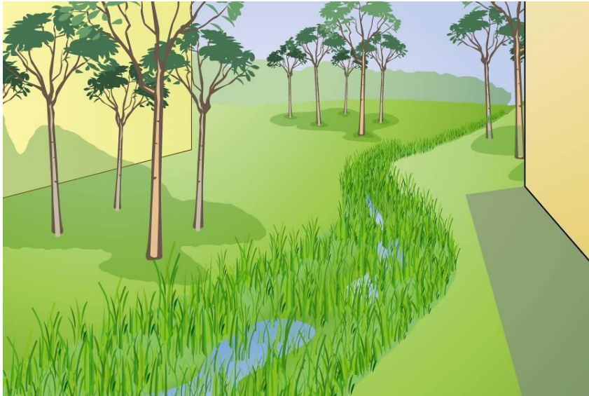
Figure 5.20. Typical Cross-section for Vegetated Swale
