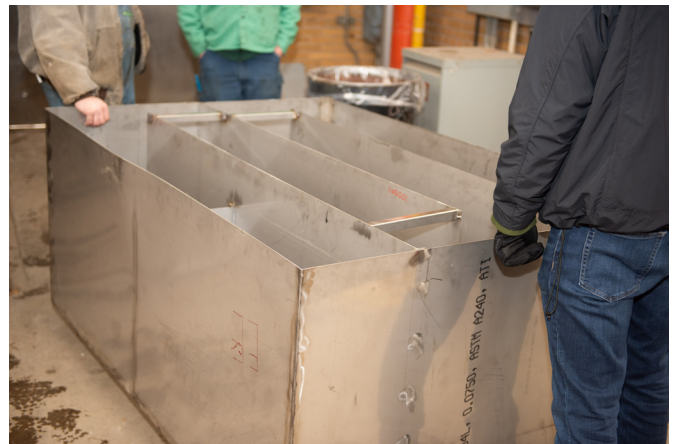
MWRD staff have designed an experimental 350-gallon tank system that could unlock remarkable potential in the biological stages of wastewater treatment to treat larger flows with less infrastructure.
