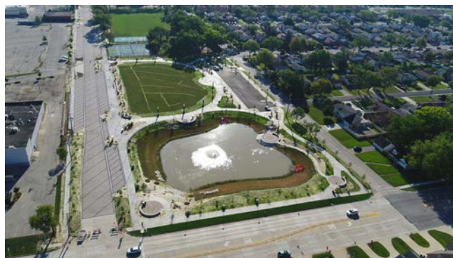
The Golf Mill Park stormwater project in the Village of Niles utilizes green infrastructure elements and permeable pavement to mitigate flooding and to improve local water quality.
