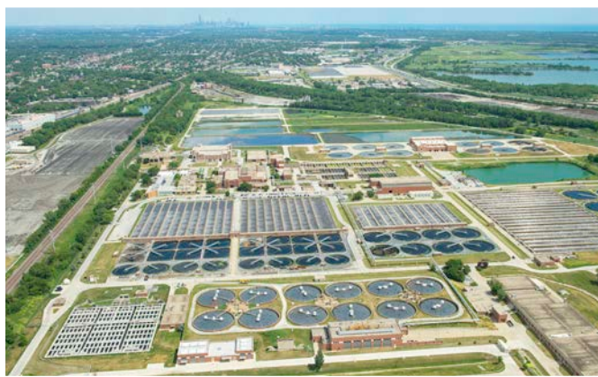
Calumet Water Reclamation Plant is the longest performing of the MWRD's seven WRPs. In operation since 1922, it serves residents and businesses in the southern portion of Cook County to clean more than 350 million gallons of wastewater per day on average. The plant's service population is more than one million people in an area of about 300 square miles.
