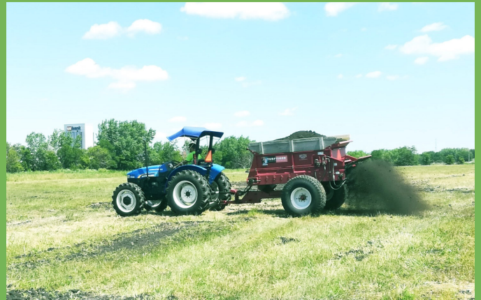
EQ biosolids prepared for incorporation into topsoil at a brownfield site (on the left) and applied as a topdressing in a grass area (on the right).
