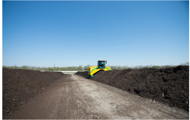
MWRD biosolids are blended with woodchips in windrow turners to create a premium quality compost product that can be used locally in gardens and lawns, golf courses, parks and fields.
