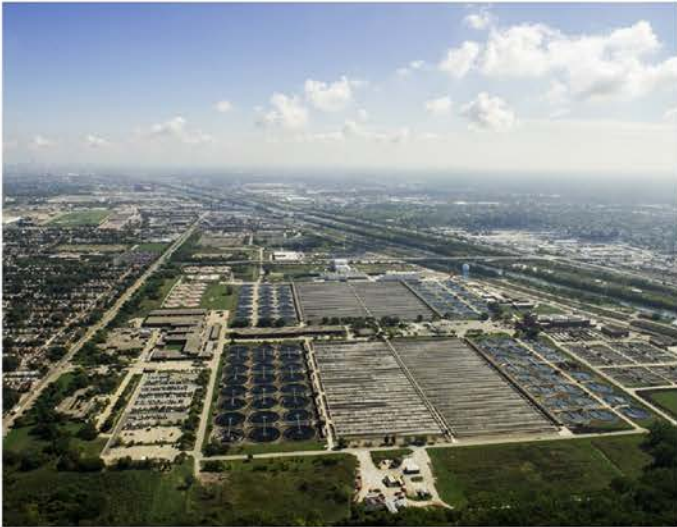
The Stickney Water Reclamation Plant remains unrivaled as the world's largest plant with full secondary treatment by volume, cleaning up to 1.44 billion gallons per day, serving 2.3 million people in a 260 square mile area.
