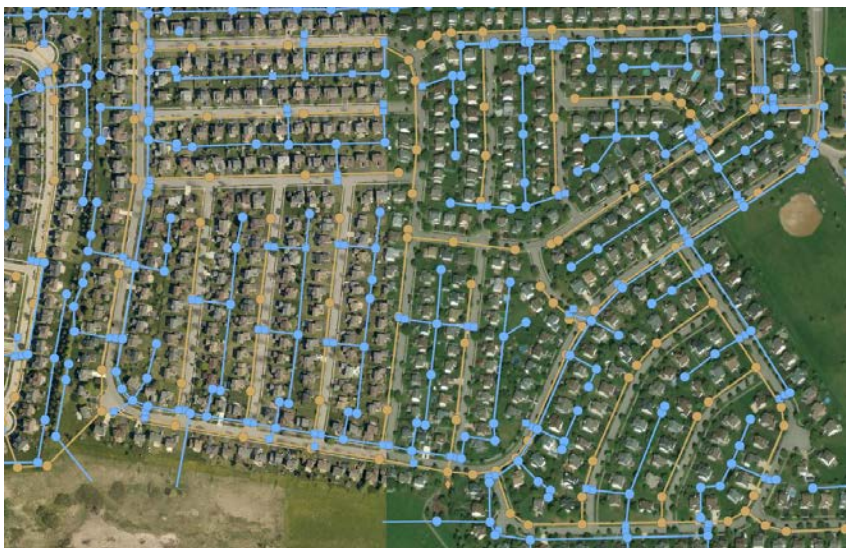
Through GIS mapping technologies and GPS units, sewer system owners can pinpoint manholes, inlets, catch basins, cleanouts, lift stations, outfalls, gravity mains, lateral lines, and other items.
