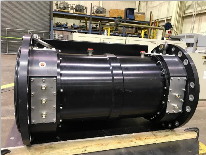
1MW permanent magnet synchronous motor
