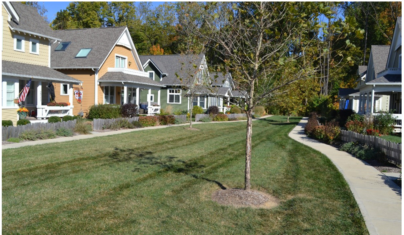
FIGURE 7.2 In a residential common area, a turf-covered trench manages runoff invisibly while preserving open space.
