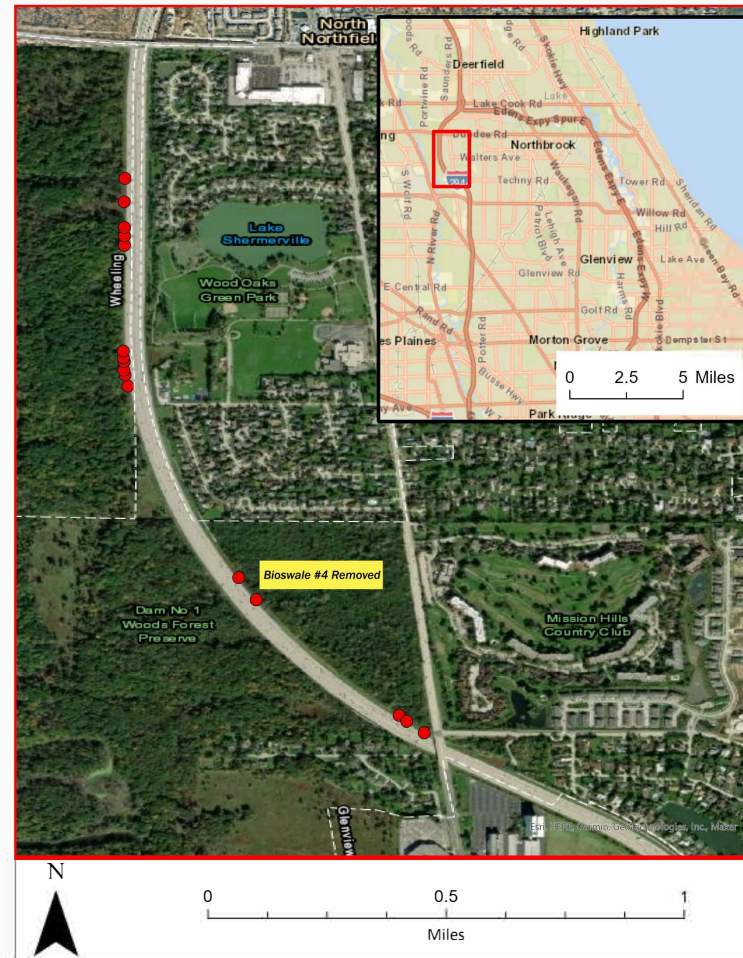
Figure 14: Bioswales selected to employ the Illinois Tollway experiment for Grant RR-22-9261. Five (5) blocked bioswales were chosen along I-294 between Mile Markers 49.9 – 51. Two (2) bioswales located northbound; Three (3) bioswales located southbound. Bioswale #4 removed due to gouged bioswale after mowing equipment accident in the plot.
