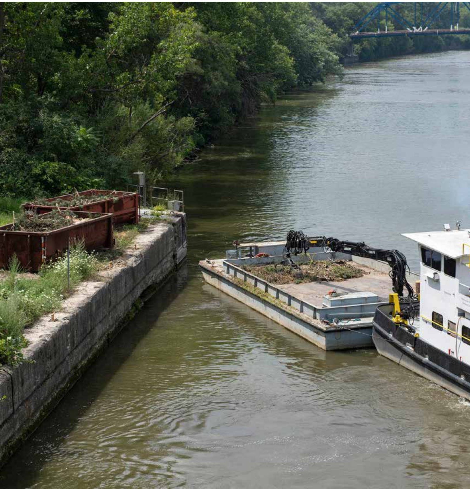
The MWRD operates a 36-foot debris boat with a 25-foot by 50-foot barge year-round for removing large logs and other heavy debris from the waterways. The boats help improve water quality and the recreational experience for thousands of boaters.
