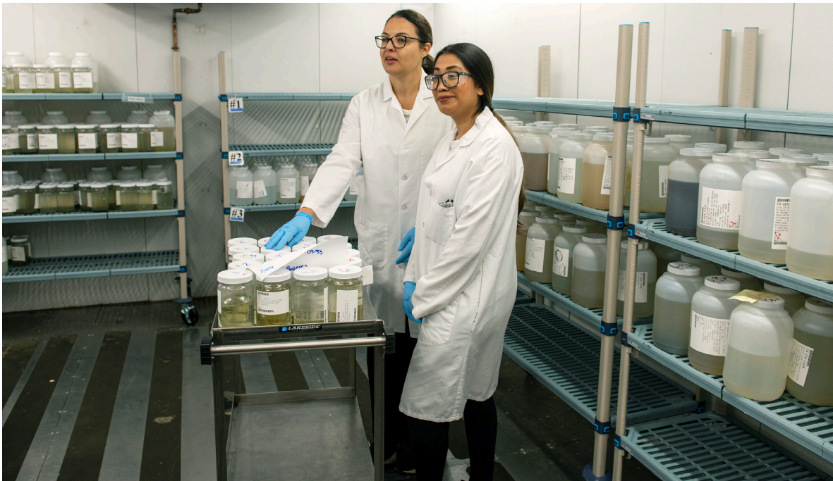
LEFT: MWRD Environmental Chemist Gosia Kokoszka (at left) and Laboratory Assistant Yolanda Izaguirre at the Stickney Water Reclamation Plant (WRP) moving samples for phenol analysis in the cooler room where samples are preserved at low temperatures until they can be analyzed.
