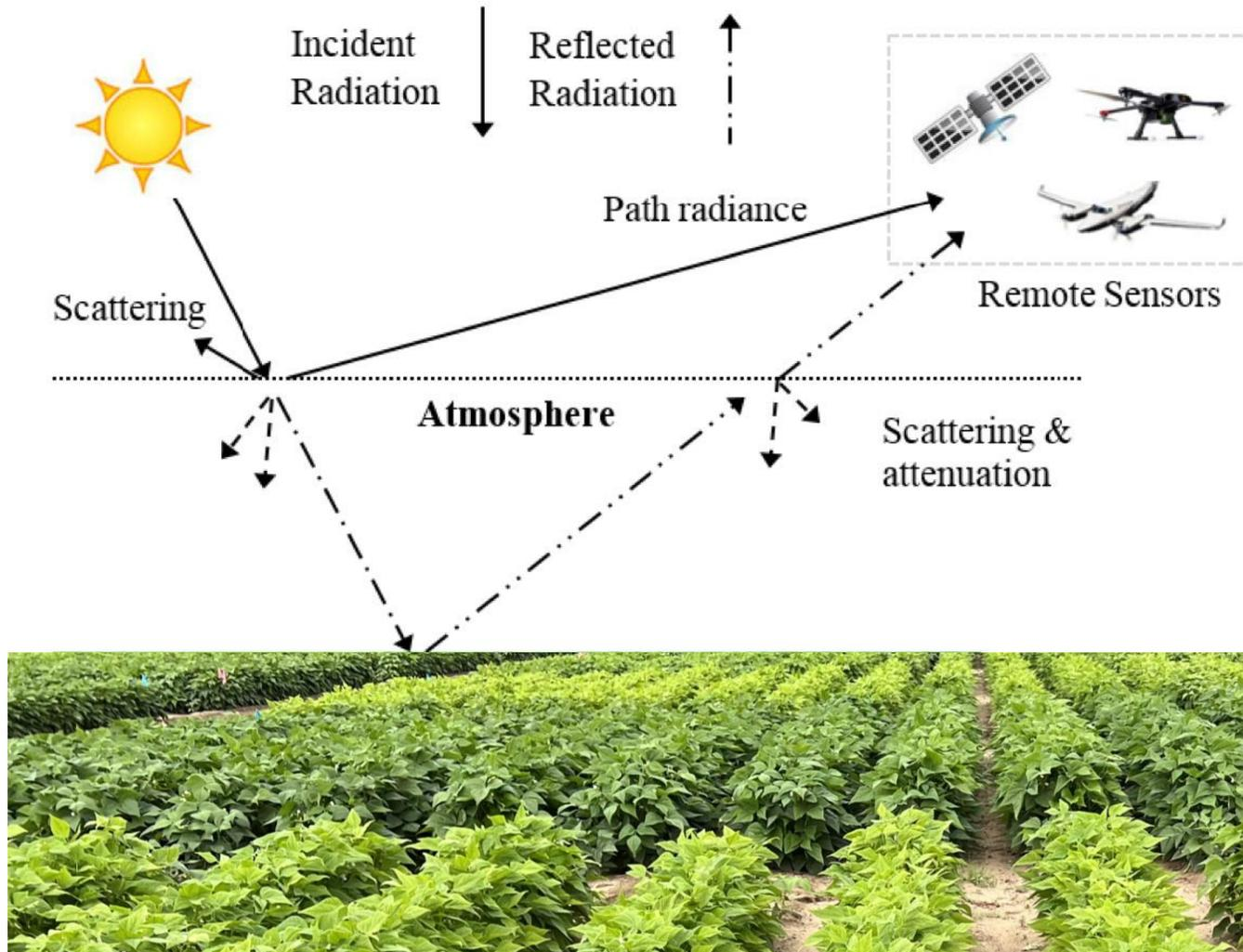
**Atmospheric effect on radiation measured by remote sensors**
