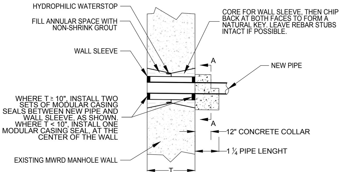
WHERE  $T \geq 10"$ , INSTALL TWO SETS OF MODULAR CASING SEALS BETWEEN NEW PIPE AND WALL SLEEVE, AS SHOWN.
