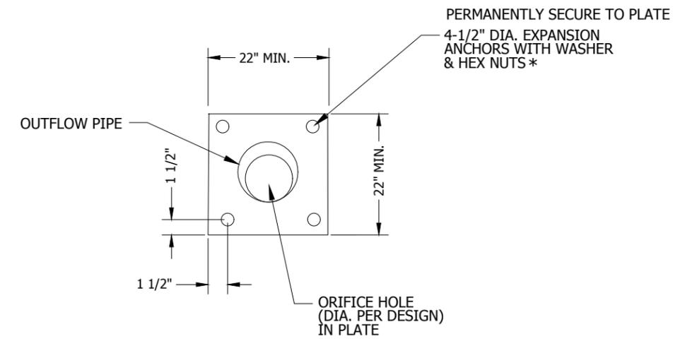
**PLATE RESTRICTOR DETAIL: ELEVATION**
