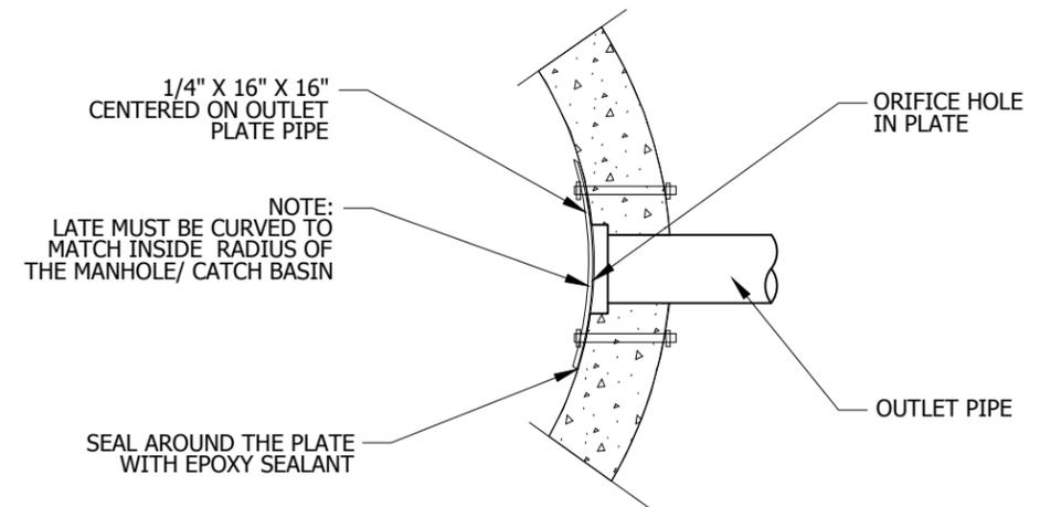
**PLATE RESTRICTOR DETAIL: SECTION**
