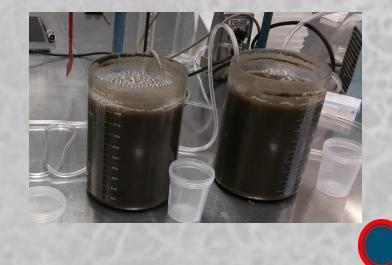
Sample from end of aeration basin, spike with phosphorus, measure uptake rate
