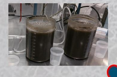
Sample from end of aeration basin, spike with acetate, measure phosphorus, then aerate to measure uptake rate
